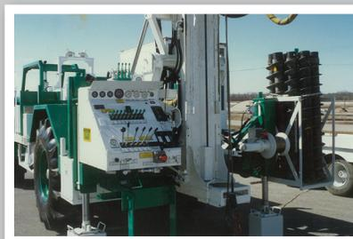
Single station control and wing around auger rack
